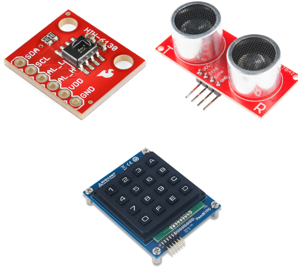
Figure 1: Temperature and humidity sensor HIH6130, keypad pmodKYPD, and ultrasonic sensor HC-SR04.
